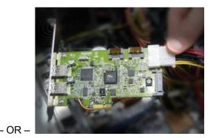
5. If you have a SATA-III hard drive or SSD, connect it to the Combo Card using the provided SATA cable. Ensure that both ends of the SATA cable are securely connected to both the card and the hard drive, and that the SSD or hard drive's power cable is also connected.
