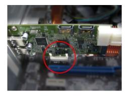
7. Secure the USB 3.0 / SATA-III Combo Card to the computer case with the appropriate screw or other mounting method used by your case.
