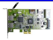
Smaller computer cases may require use of the included Low Profile Bracket in order to install the Expansion Card in your system. Unscrew the two mounting screws as shown, then position the Low Profile Bracket onto the card and reattach the screws.
